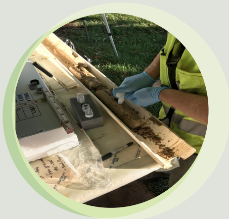
Soil samples are tested to identify contaminant release sites
