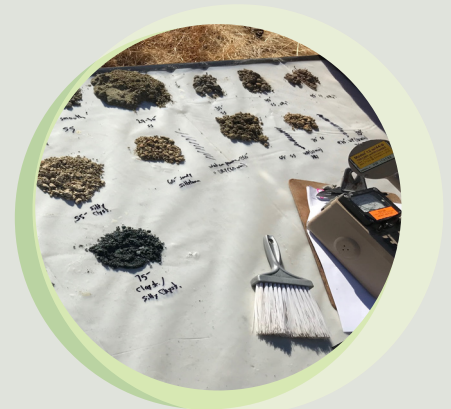
Analyzing logging drilling cuttings to understand the geology beneath Site 300
